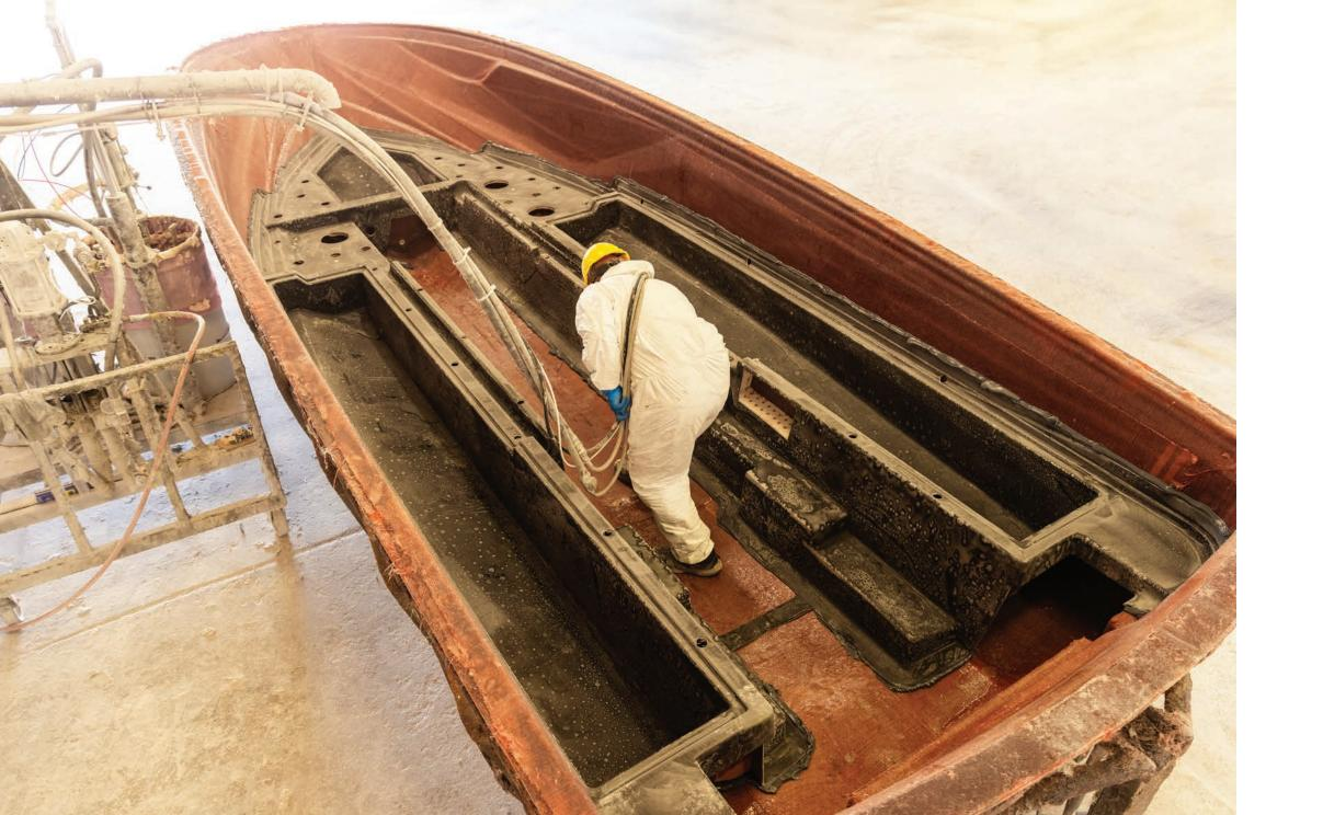
LEFT: A Centurion has strength at its core with a specifically designed stringer system that houses as much as 3350 pounds of ballast and welcomes six stable mounting points for a PCM engine.
