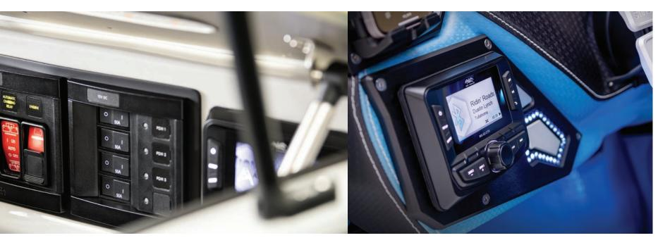
ABOVE: Conveniently accessible battery management is another user inspired innovation from Centurion. We have transformed the isolator switch buried in the observer's storage area into a truly isolated system conveniently located in the glovebox next to a PDM switchpanel for troubleshooting. **OPPOSITE:** A Centurion Ri Series driver benefits from the coolest toys. The Lit shifter and lighted Centurion badge at the throttle console, proves, "He who drives the coolest toys, wins."
