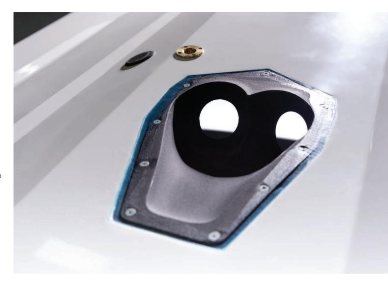
LEFT: Centurion's RAMFILL<sup>2</sup> scoop is located just in front of the engine. Both of the filling 2" stainless steel ball valves can be opened to allow as much as 2900 pounds of water to fill the sub-floor lounge tanks in 90 seconds at 14.9 miles per hour.
