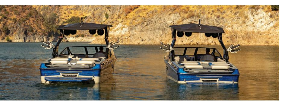
ABOVE: As much as 5850 pounds of ballast displaces the hull 10 inches farther into the water to generate the waves and wakes Centurion is known for. There is no replacement for displacement. **OPPOSITE:** The locations of Centurion's ballast are distributed evenly throughout the boat to displace the entire running surface and create a longer, pushier wave. This balanced approach to weight distribution also eliminates bow rise allowing the boat to operate more efficiently.
