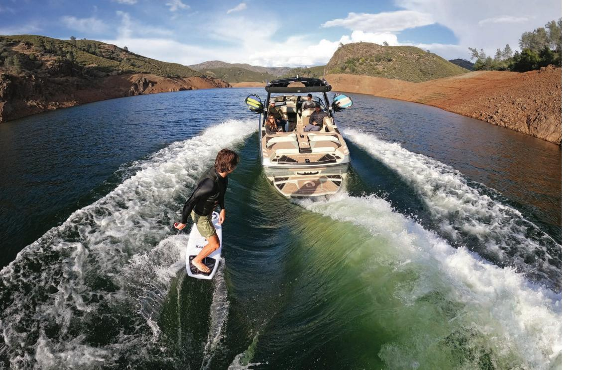
LEFT: Ballast and passenger weight can be evenly distributed in a Centurion to achieve a professional level surf wave with the help of QuickSurf Pro. QSP creates lift opposite the surf side to displace the surf-side corner slightly more and create the curl.
