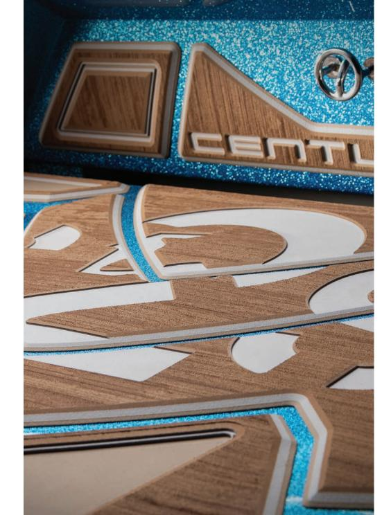
LEFT: Centurion vinyl is made by Spradling with a 17 mil top coat to guard against staining and abrasions. This vinyl is sewn together with Teflon thread in seams of double and triple stitching. There are no corners cut or steps skipped when crafting a Centurion interior built to last.
