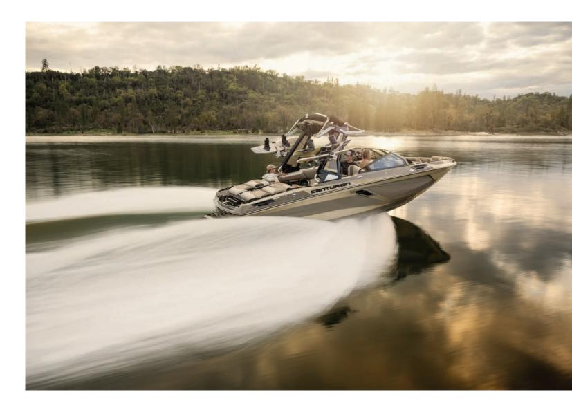
LEFT: This 2025 Centurion Ri265 demonstrates the smooth ride of the Opti-V Hull. The deep-v of this hull cuts through the chop and absorbs the shock of a rough water ride.
