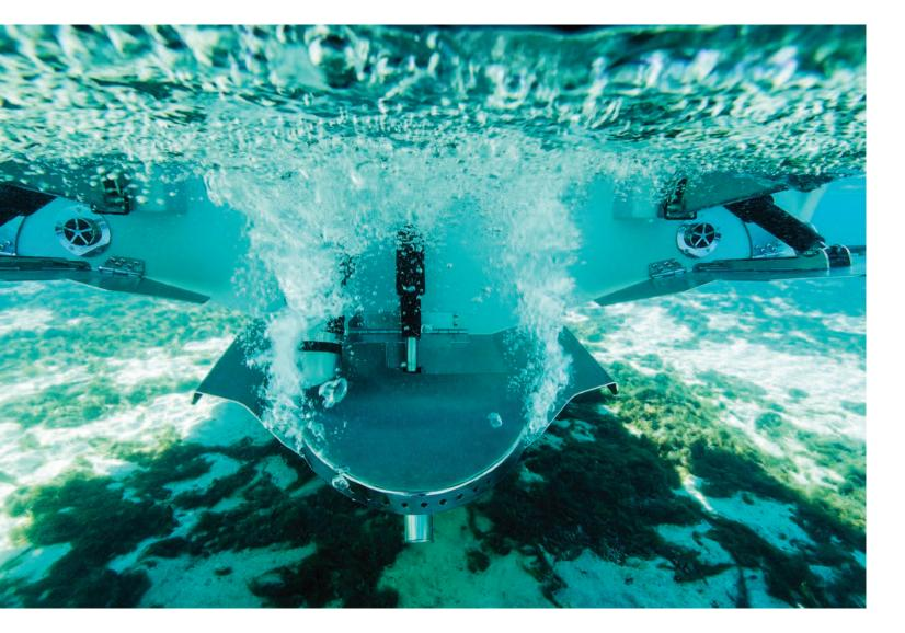
LEFT: The Silent Stinger Wake Plate is a trim tab that adjusts your attitude. Not only does it change the running attitude of a Centurion, it also changes your attitude on the water by keeping the engine noise inside voice quiet.
