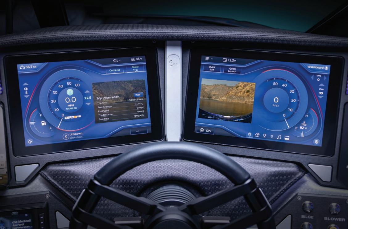
LFFT: The Range of View (ROV) system includes front and rear facing cameras along with a detailed look into real time trip and fuel usage data. Standard on the Centurion Ri Series, the ROV allows the driver to see in front, behind and inside simultaneously for a range of views.
