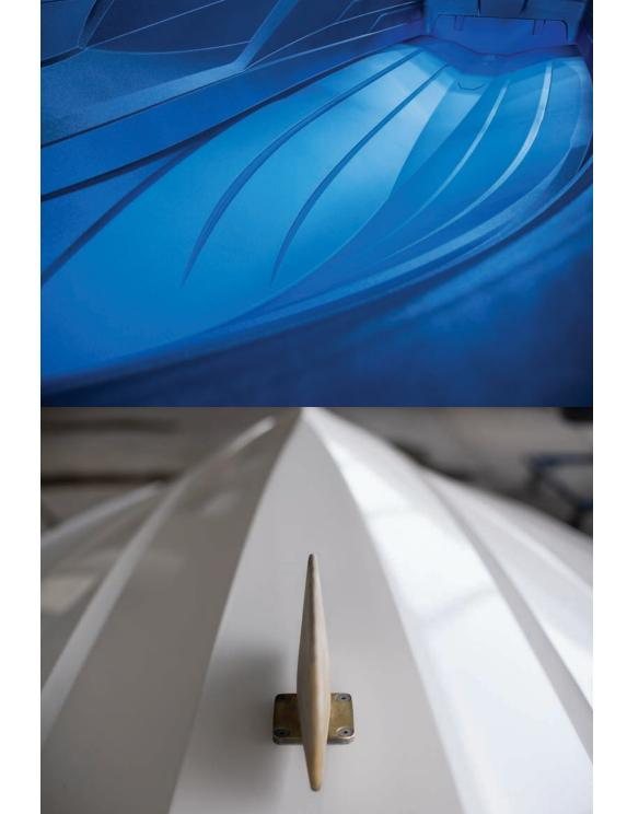
LEFT TOP: This is a Centurion Ri hull mold between color sprays during the Gel Coat process.
