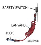
The engine emergency stop switch is an extremely important safety precaution. Use the engine emergency stop switch when operating the boat's engine. This safety device prevents your boat from becoming a runaway if you are accidentally thrown from the seat or away from the helm.
