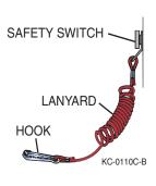
The engine emergency stop switch controls the engine ignition ON/OFF. This safety device shuts the engine off immediately and prevents the boat from becoming a runaway if the operator is accidentally thrown from the seat or away from the helm.
